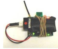
Fig. 15. This small lightweight footstep detector is designed from the schematic level on up using the WARPWING system as a base, but replacing the accelerometer with one far more sensitive.
