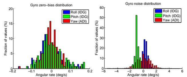
Fig. 4. The variation of the gyro zero-bias for a single board across 150 runs over 5 days is shown in the graph on the left for each of the three axes. The graph on the right shows the zero-rate gyro outputs over 2000 measurements during a single run. The bias offsets are clearly visible in the right graph, as well as a notable difference in performance between the two gyros.
