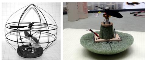
Fig. 12. The hopping rotochute developed at GATech uses WARPWING as its flight controller. The software interface was rewritten to fit in to the existing MATLAB framework, while the rest of the WARPWING system remained unchanged. This allowed for quick development of the mini rotochute, shown at right.
