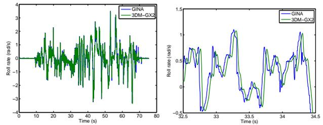
Fig. 6. Comparison of gyro output between GINA and 3DM-GX2
