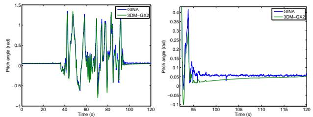
Fig. 9. Pitch angle estimate comparison. The noisier GINA estimate also allows a much shorter settling time than the 3DM-GX2.
