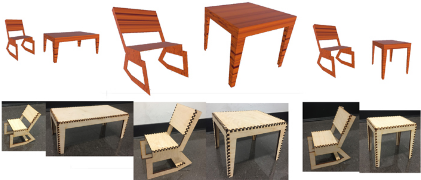
Figure 9: From the creations of the ten non-designer participants that attended our design session, we selected six furniture designs participants had made, and manufactured 1/8 scale models.
