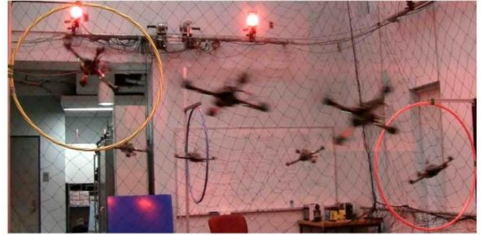
Fig. 7. Composite image of a single quadrotor quickly flying through three static circular hoops. See attached video or http://tinyurl.com/pennquad .
