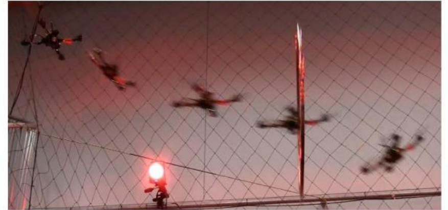
Fig. 5. Composite image of a single quadrotor flying through a thrown circular hoop. See attached video or http://tinyurl.com/pennquad .
